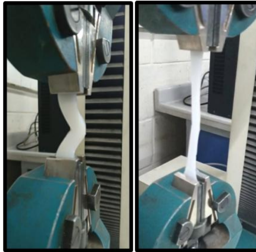
Figure (7): tear strength specimen during mechanical measuring
