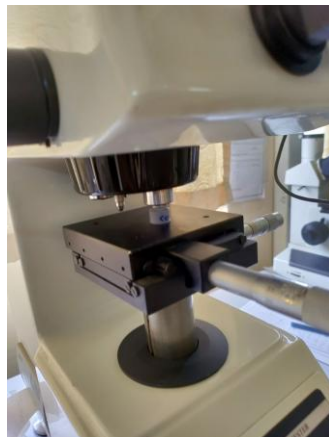
Figure 4. Vickers microhardness testing device applying a controlled load via a diamond indenter to evaluate the surface hardness of monolithic and multilayer zirconia specimens.
