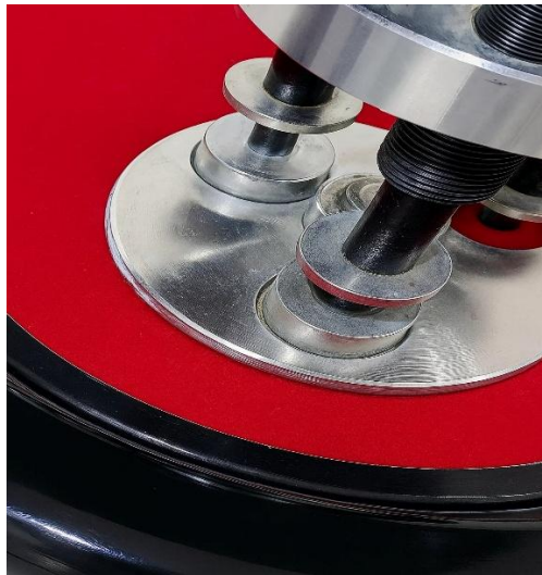
Figure 3. Close-up view of the polishing head applying consistent vertical load to the specimen holder, enabling reproducible and uniform surface finishing across all samples.
