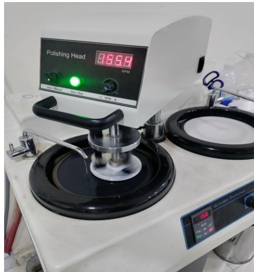
Figure 1. Dual-disc semi-automatic grinder–polisher equipped with independent pressure heads, utilized for standardized surface preparation of zirconia specimens before testing.
