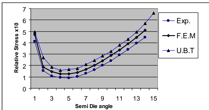
Fig.(7). Relationships between semi die angle & Relative Drawing stress in friction (Am= 0.05) (Comparison with U.B.T & Exp results)
