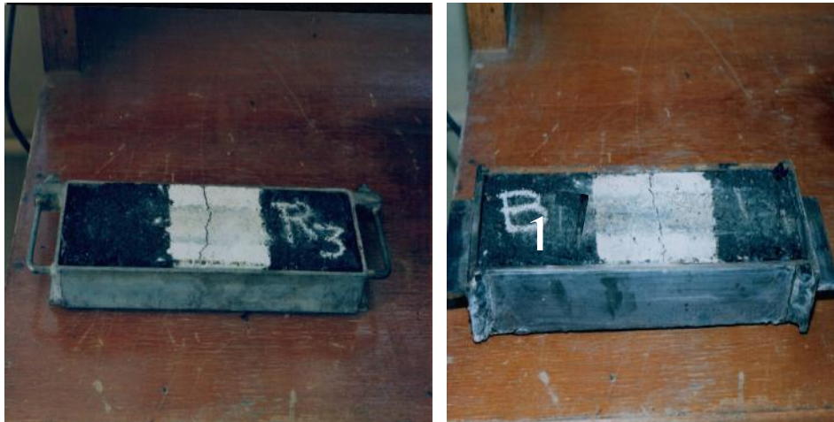
Plate (3):- Propagation of Reflection Cracks
