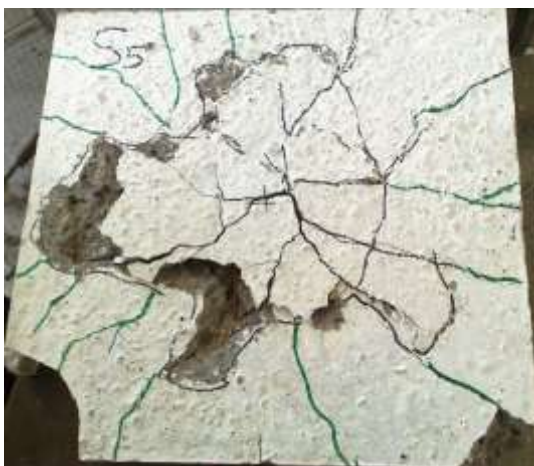
Fig.(19)Crack Pattern at Failure for Specimen S5.
