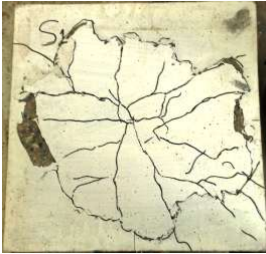
Fig.(15) Crack Pattern at Failure for Specimen S1.
