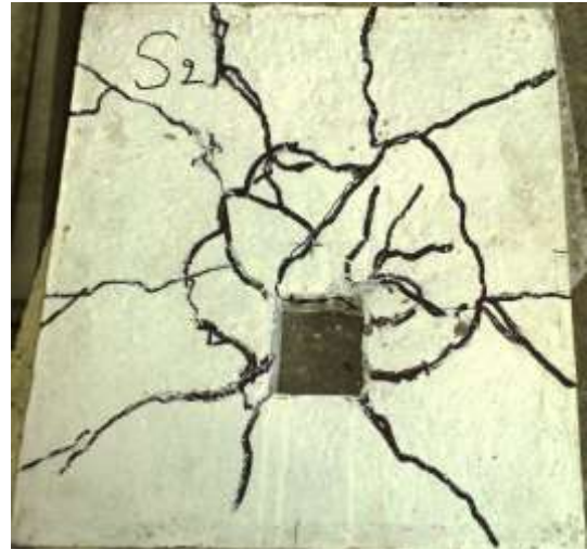
Fig.(16) Crack Pattern at Failure for Specimen S2.
