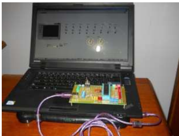
Figure (20): Proto type data acquisition card
