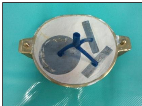
Figure 2. Metal mold with wax sprue for Valplast denture base material.
