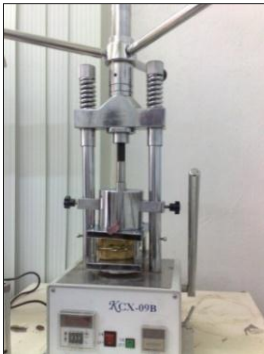
Fig 3. Manual injection unit for Valplast denture base material
