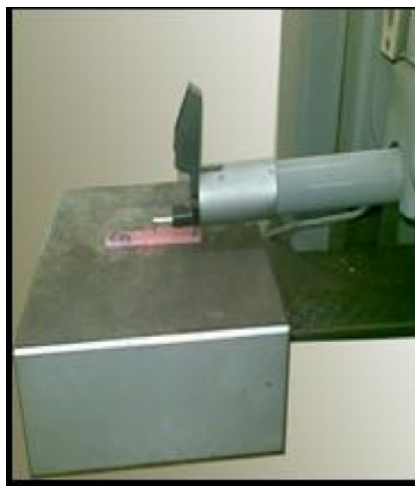
Fig 4. Profilometer device for surface roughness of denture base material.
