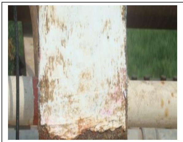
Fig. (6): Growing of Barnacles on uncoated portion of model after immersed in Shat-Arab river at Al- Asharlocation
