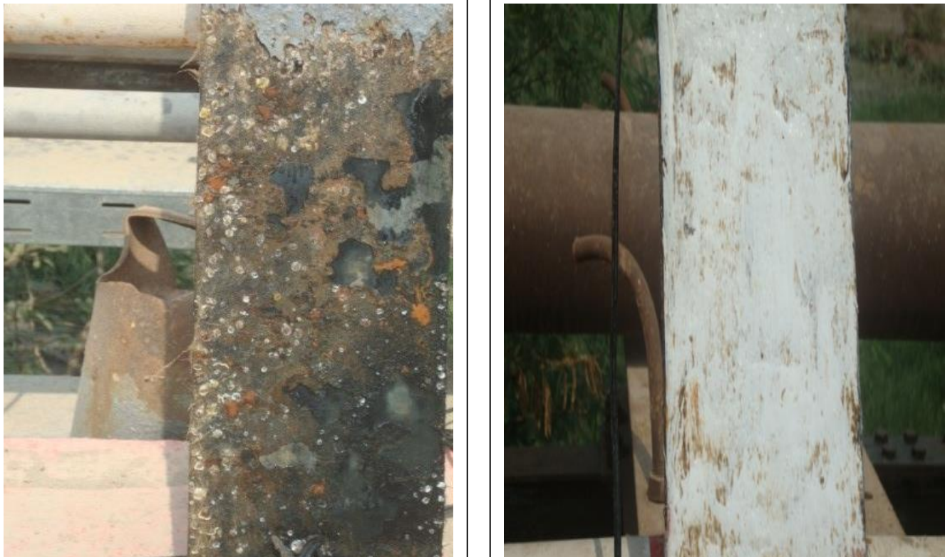
Fig. (7): Growing of Barnacles on uncoated portion of model after immersed in Shat-Arab river atFaolocation
