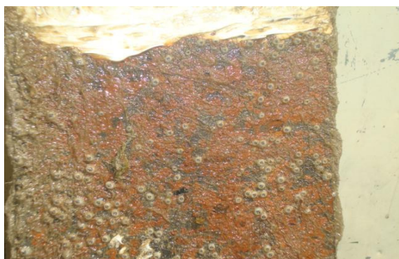
Fig. (6): Growing of Barnacles on uncoated portion of model after immersed in Shat-Arab river at Al- Asharlocation
