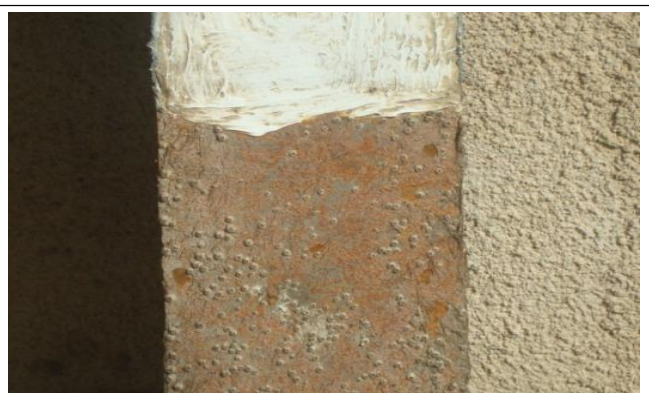
Fig. (6): Growing of Barnacles on uncoated portion of model after immersed in Shat-Arab river at Al- Asharlocation
