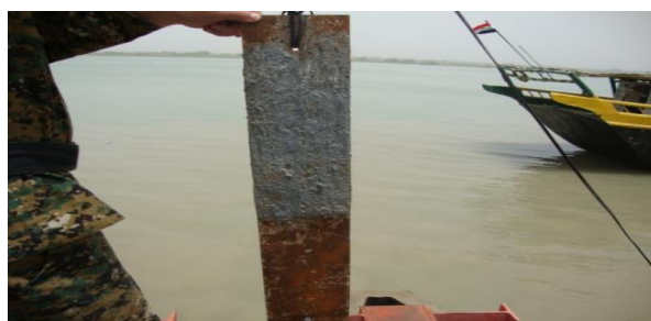
Fig. (5): Immersion of Model in Shat-Arab river at Fao location
