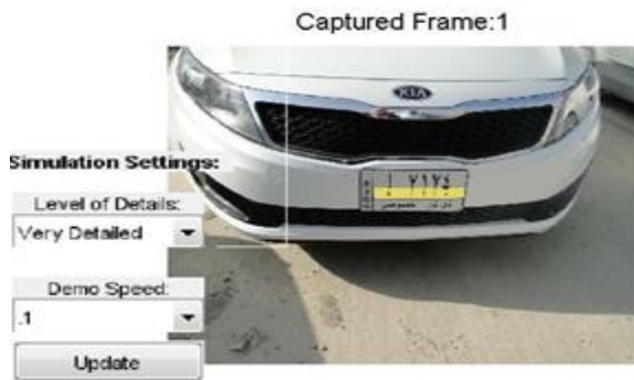
Determining the angle of the plate using the Radon transform:
